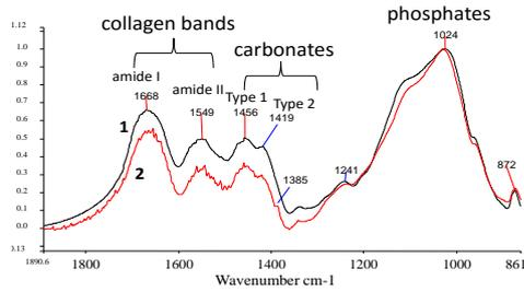
**Figure 1:** FTIR spectral region containing amide I, II, carbonates and phosphate groups of artificially aged bone sample.
